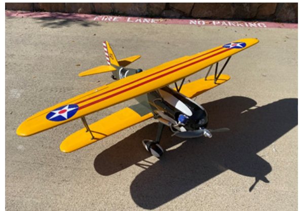
Great Planes P6E Hawk RTF minus RX, Magnum 52 Four stroke, Extra Cowl
